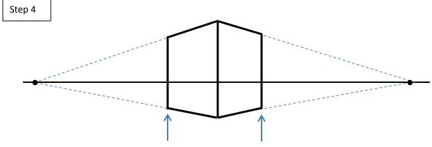
Draw the vertical lines that are parallel to the center vertical line to complete the sides of the building.
